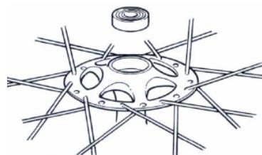
3. Having noted the correct orientation of the axle, insert it in place from the left hand side of the hub until the axle's 'shoulder' butts up against the bearing unit.
