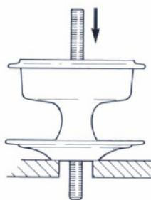
2. With the axle removed, invert the hub shell and drive out the L.H. bearing using an 11-12mm drift (or old axle).
