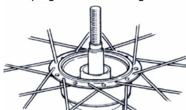
4. Slide the left hand bearing unit into place and press home using a suitable punch exerting pressure across the full face of the bearing unit whilst supporting the right hand bearing across the full face.
