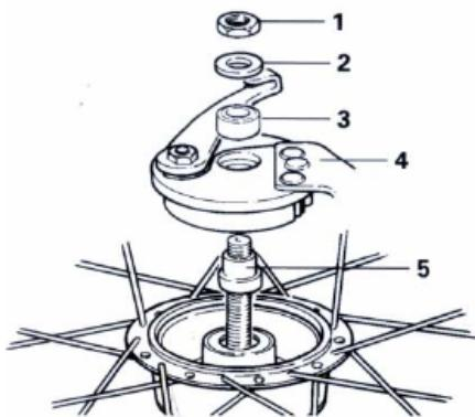
3. Clamp L.H. end of axle in vice and remove R.H. locknut and spacers (you may also have to remove the freewheel screwed on X-RD).
