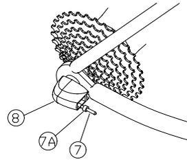
7. Connect the indicator (7) to the cable connector (9). If you do not have a pre-assembled cable connector, take the cable anchorage (10) instead and see step 7.1 and 7.2.
