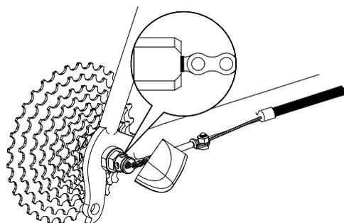
3. Tighten the indicator locknut (7A) to lock in adjustment.
