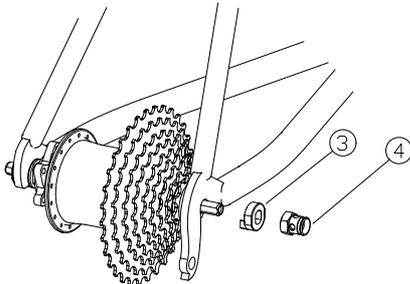
4. Fit the lock-washer (3), dome nut (5) on the left side of the axle. **Screw the nut finger tight.**
