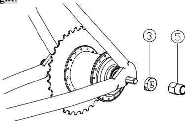
5. Align the wheel. Tighten the guide nut and dome nut to **28Nm**.
