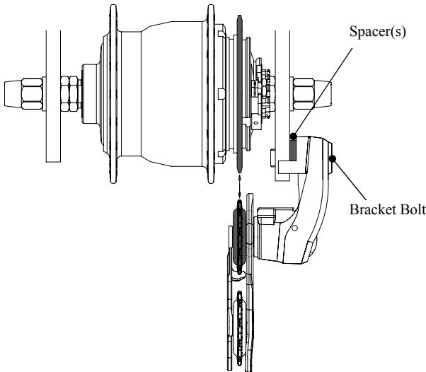
The total thickness of spacer(s) used should not exceed 8mm.
