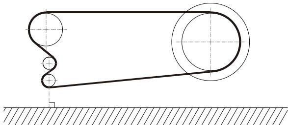
If the difference in teeth number between the largest and smallest chainring is 13T-16T, make the chain one link longer than this.
