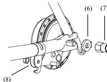
Fit proper lockwashers according to dropout type.
