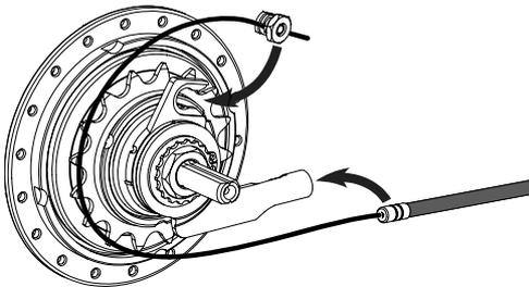
There is an auxiliary hole by the groove. You can insert a 2mm Allen key or a #14 spoke in the pulley and then turn the pulley clockwise to help fit the cable-anchorage unit.
